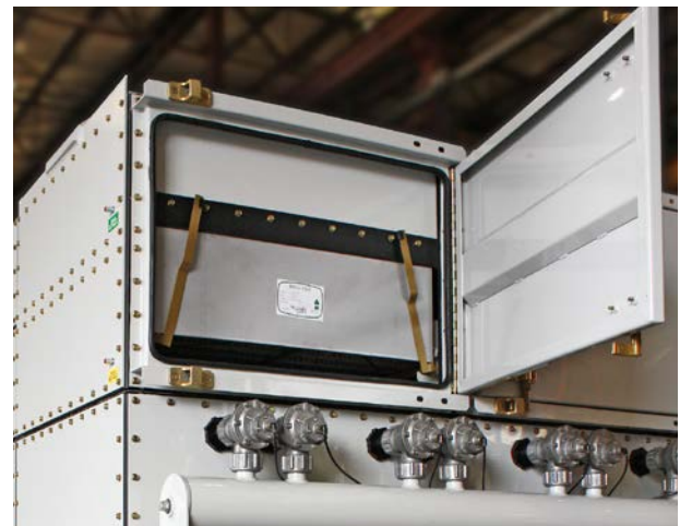
This integrated safety monitoring filter prevents collected dust from re-entering the workspace if there should be a leak in the dust collector's primary filtering system.
