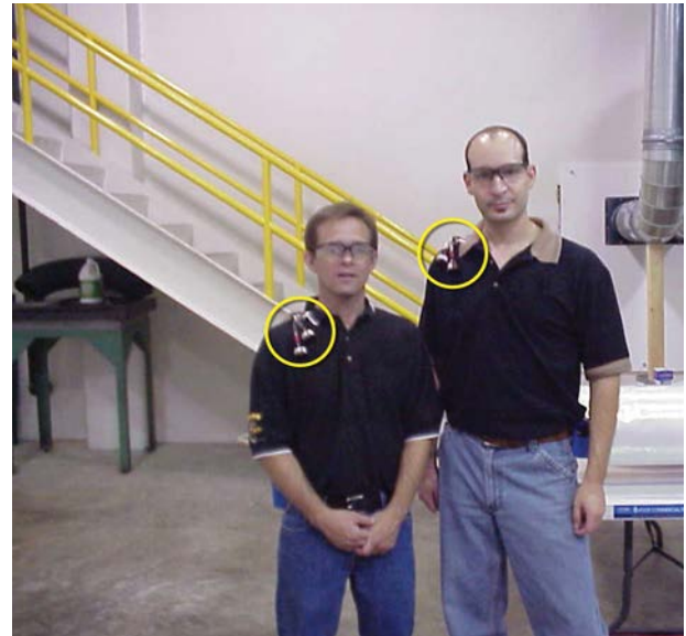
Air sampling pumps and filters worn by workers in an emissions test are used to monitor indoor pollutant levels to determine whether the shop is in compliance with OSHA.
