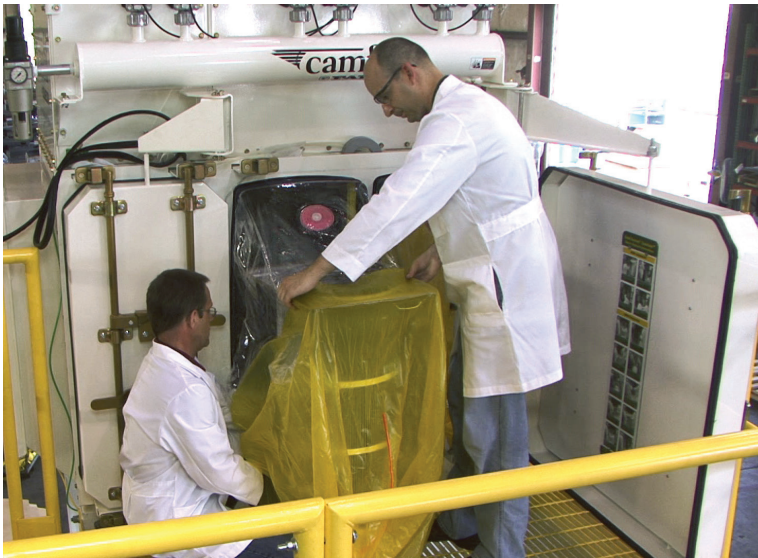
Example of a surrogate tested “bag in, bag out” safe change filter option for a dust collector
