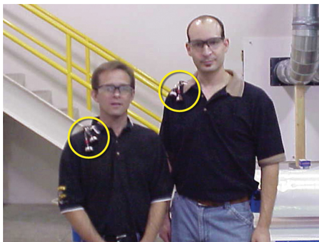
To monitor air quality, workers wear a small air pump and filter attached in the breathing zone.
