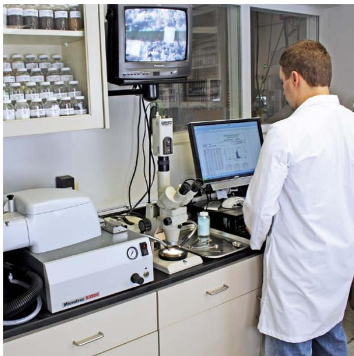
*Bench testing identifies physical properties of the dust, aiding filter selection.*
