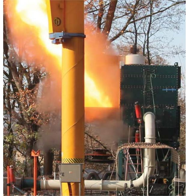
*An engineered test is performed at an official testing facility to confirm that this dust collector can withstand an explosive event. Scan QR code to view brief explosion test video.*
