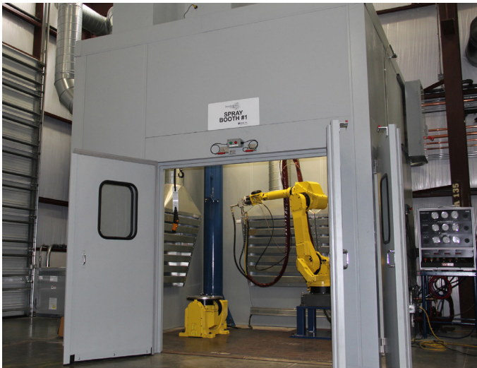
HVOF and plasma spray booth with dust collection.
