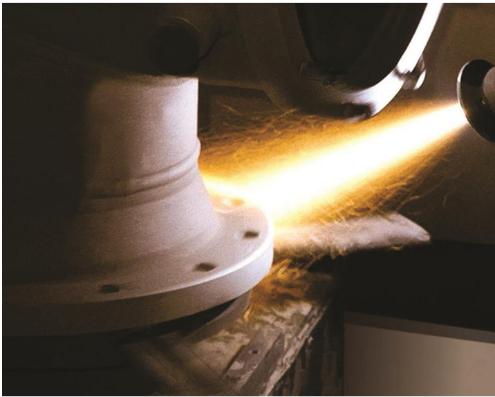
Wire arc spray process.
