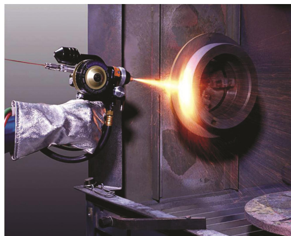
Combustion wire spray process
