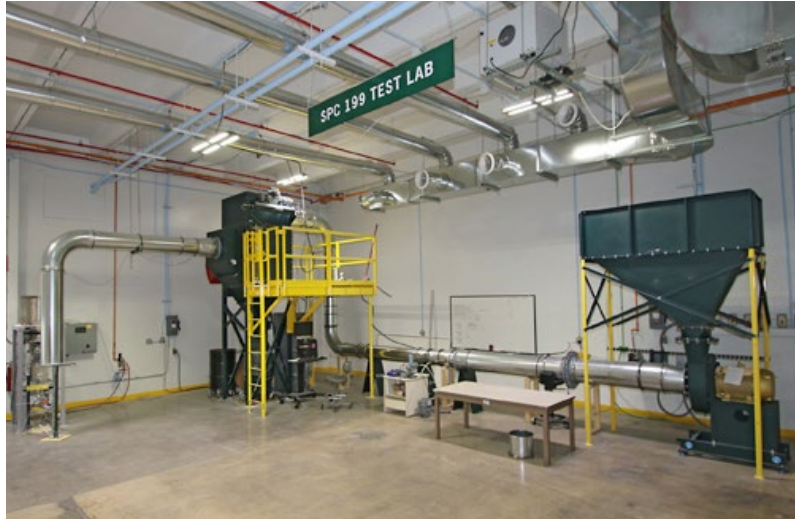
Full-scale test rig in the Camfil APC laboratory has been built in accordance with Standard 199 specifications. It is used both in the company's internal testing and for customer assistance.
