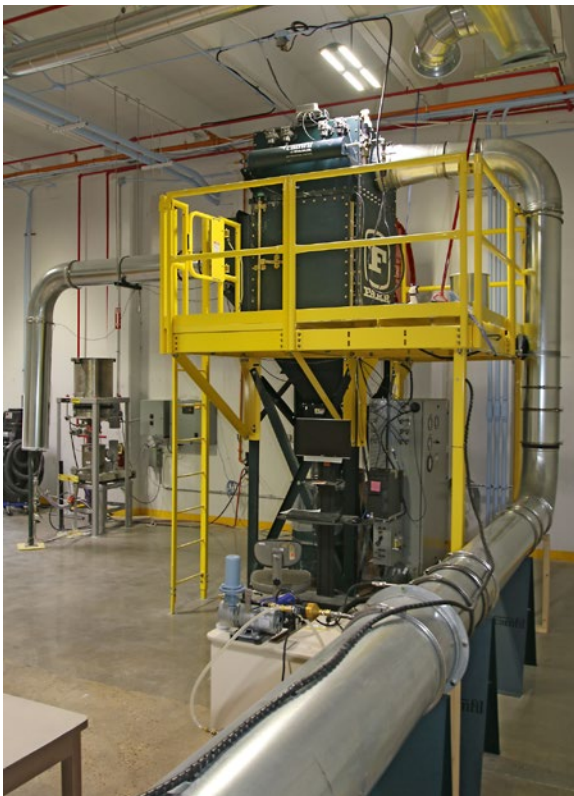
Using a cartridge dust collector with four high efficiency filters, the Camfil APC test rig feeds dust into the collector under conditions specified in Standard 199.
