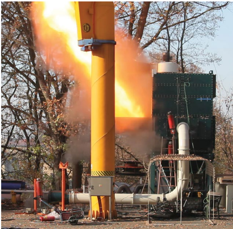
Combustible dust explosion hazards must also be evaluated when designing a dust collection system. Photo shows a controlled explosion staged to test how this collector will hold up in a combustible dust event.
