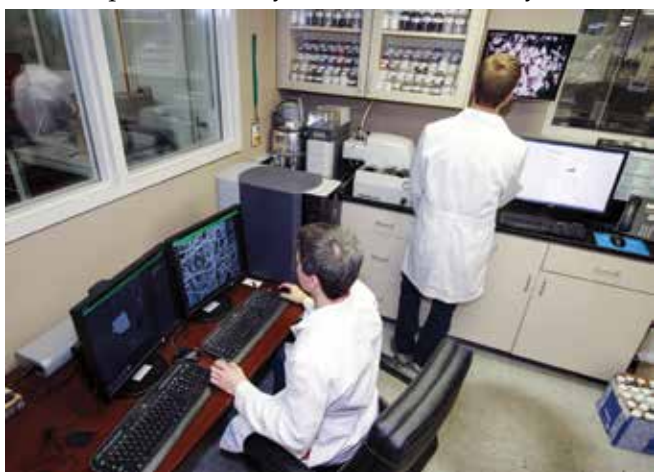
Test lab workers perform dust analysis to identify particle characteristics relevant to selecting the correct filter media.
