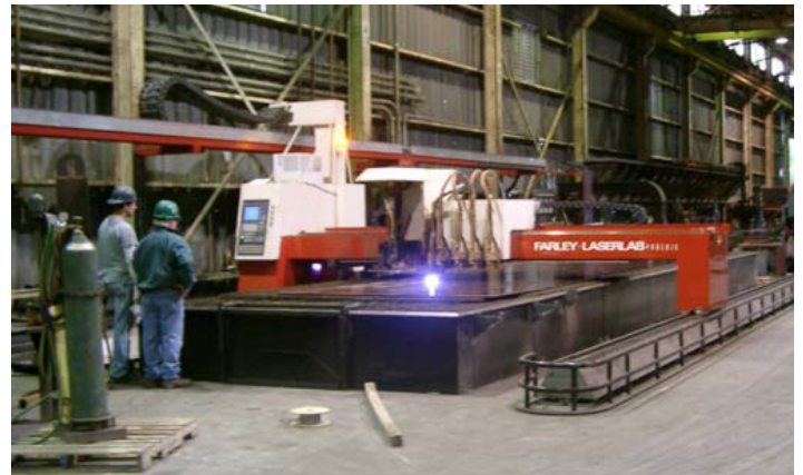
After Farr Gold Series collector was installed plasma smoke is well controlled, maintaining clean operating conditions and ensuring worker safety.
