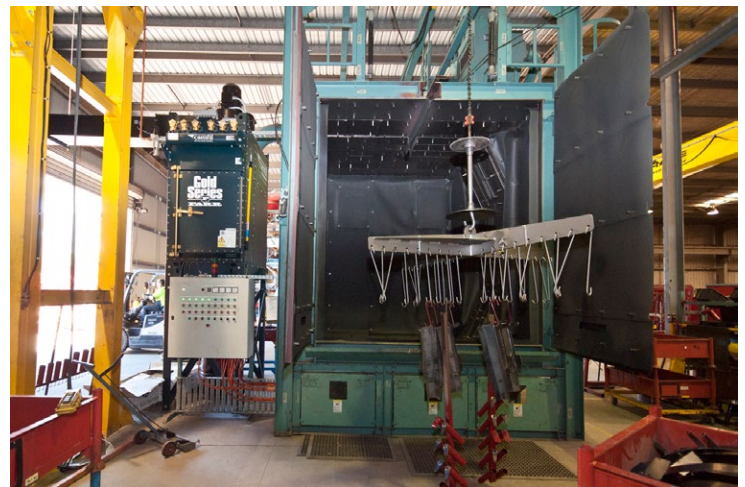
▲ The ABSS Spinner Hanger machine includes high throughput with optimum blast coverage.
