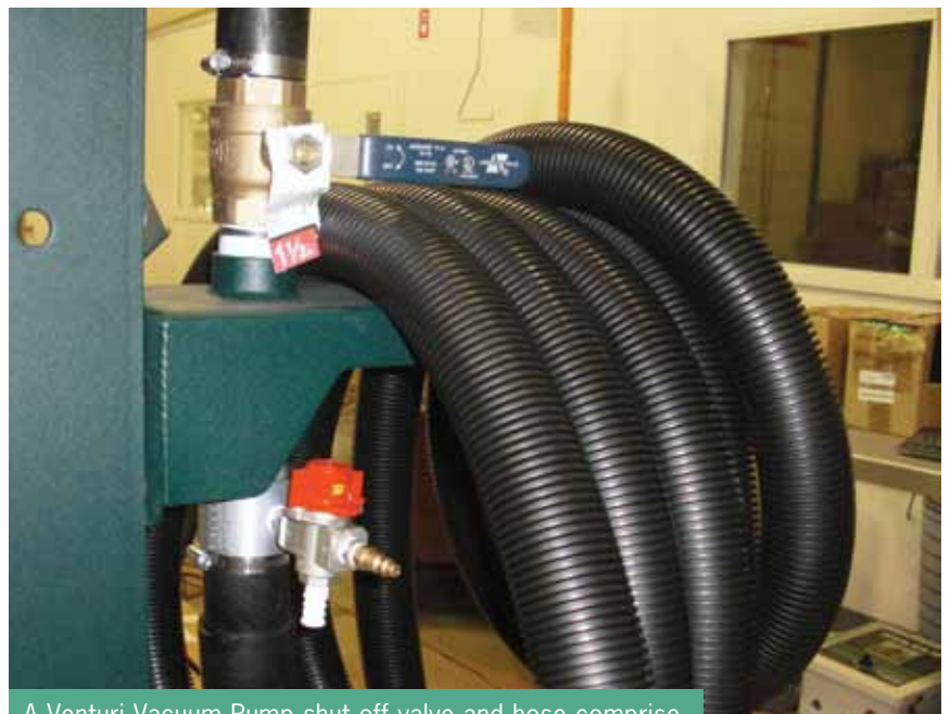
A Venturi Vacuum Pump shut off valve and hose comprise the Clean Sweep system.
